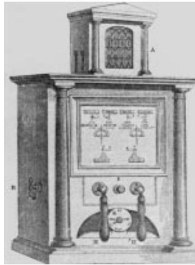
Fig. 3. Double-needle telegraph of Cooke and Wheatstone, which was used in England in the 1840s. [From *Engineers & Electrons* by Ryder and Fink (Piscataway, NJ: IEEE Press, 1984)].
